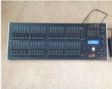
Current lighting desk is very simple and would not work with modern LED lighting or moving fixtures
